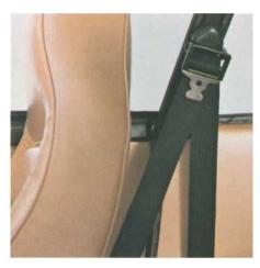
Three-point retracting seat belts are standard for the bucket seats. When the car is in use, seat belts should never be found in this position.
