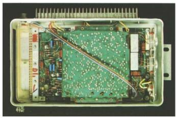
The computer has electronic sensors that monitor air and coolant temperature, air pressure, rpm's and throttle position. From these five readings, the computer determines what precise quantity of fuel should be injected into the cylinders. And orders it injected.
